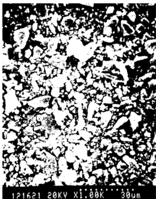
Fig. 2. Scanning electron micrograph of \text{ZrO}_2 particles for the w/o volume ratio 5/100 when \text{Zr}^{4+} concentration is kept 1 M. The other operation conditions are the same as in Table 2.
